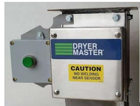
Figure 11 - Calibration button install
