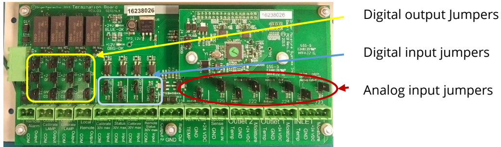
Figure 33 - I/O board jumper location
